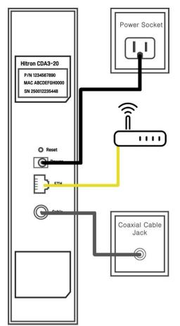
After few minutes of waiting on signal, Power, Down Stream, Up Stream and Online must be steady on. If any of top 4 lights are missing or flashing, please contact us at <a href="mailto:support@gtatel.com">support@gtatel.com</a> for further assistance.
